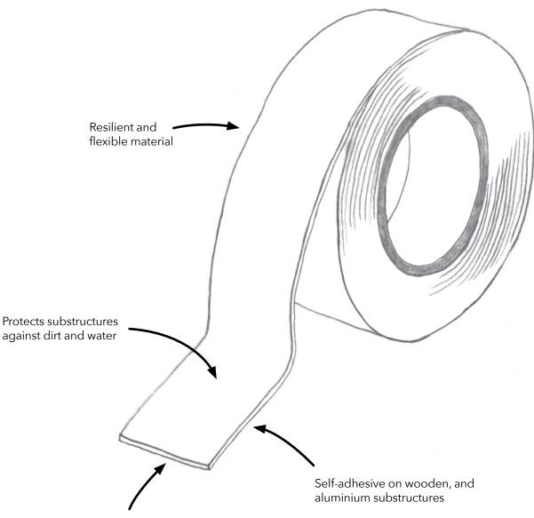
Separates surface friction between a concealed connector and the substructure
